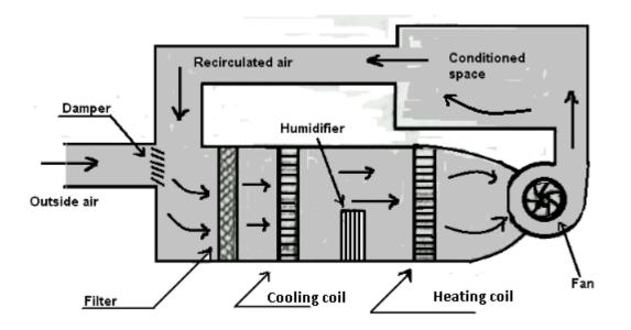
In summer air conditioning system, the cooling by operates to cool the air to the desired valve. The dehumidification is obtained by operating the cooling coil at a lower temperature than the dew point temperature.
