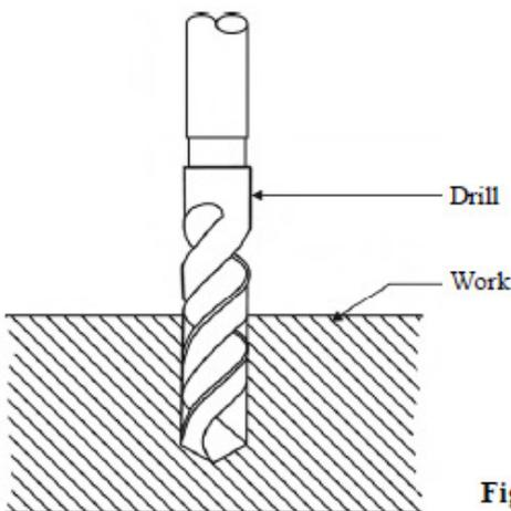
Fig 2.17 Drilling
