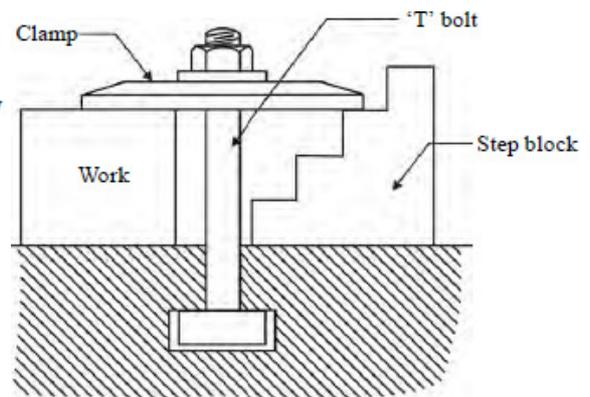
**Fig 2.7 T-bolt & clamp**
