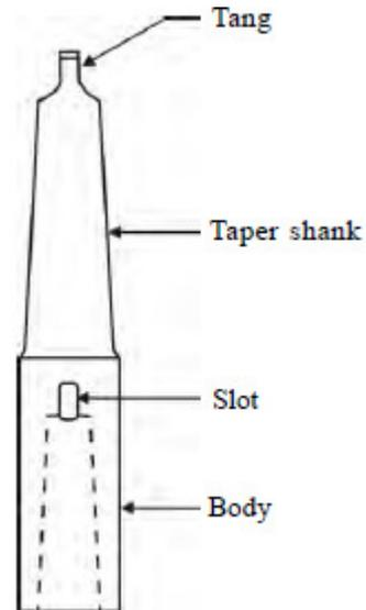
Fig 2.14 Drill socket
