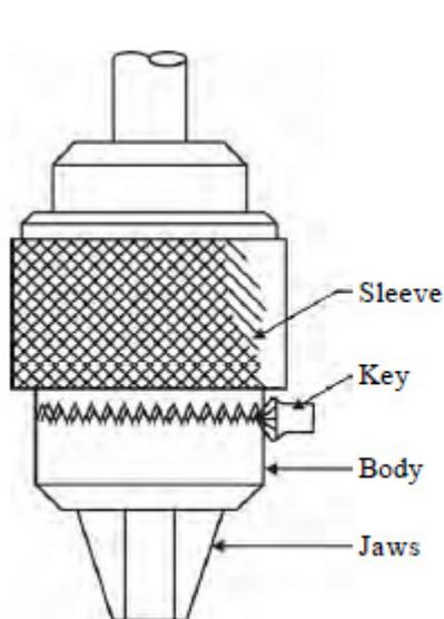
Fig 2.15 Drill chuck
