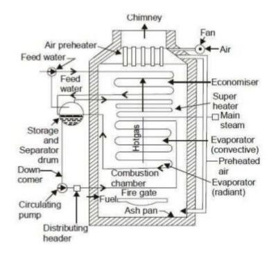
This boiler works on basic principle of forced convection. If the water is circulating by a pump inside the tube, the heat transfer rate from gas to the water is increases. It is the basic principle of it.
