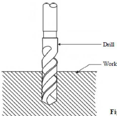
Fig 2.17 Drilling
